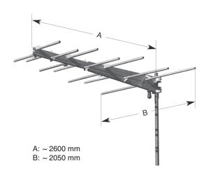
Hot-dip galvanized steel. Material:
